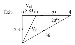
In the opposite direction of  $V_{u1}$  hence addition  $P = 900 \times 25 (65 + 8.83) = 1.661 \text{ MW}$
