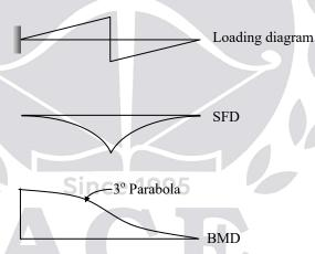
Slope of SFD = Rate of loading and
