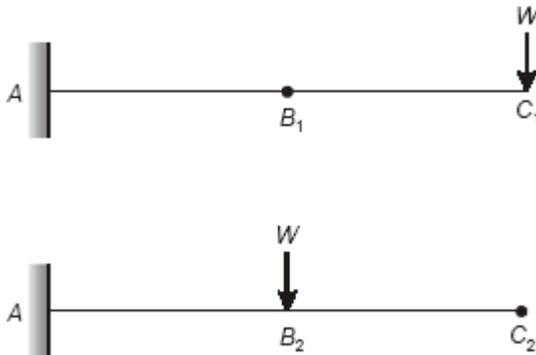
So, the ratio of deflection at point  $B_1$  due to load at  $C_1$  to the deflection of point  $C_2$  due to load at  $B_2$  is \_\_\_\_\_.
