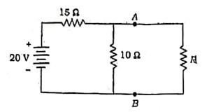
What should be the value of resistance R in the above circuit, if it has to absorb the maximum power from the source?
