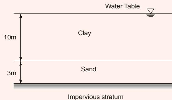
The settlement (in mm, round off to two decimal places) of the clay layer, 10 years after the construction of the fill, is \_\_\_\_\_.
