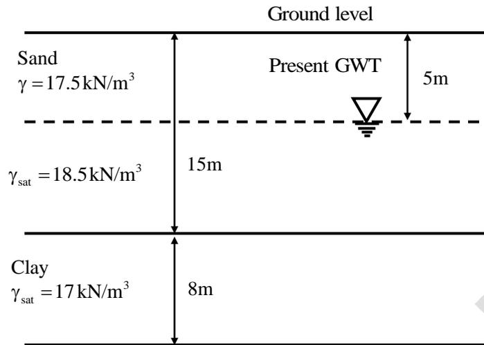
The over consolidation ratio (OCR) (rounded off to two decimal places) at the mid-point of the clay layer is \_\_\_\_\_.
