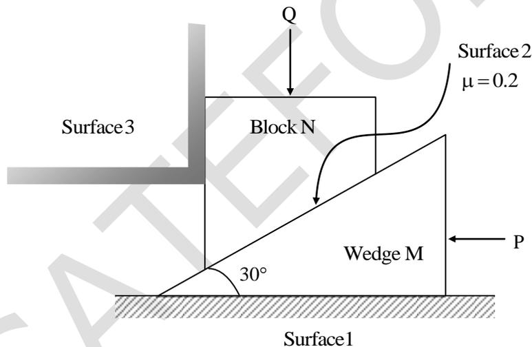
If force P is sufficiently large, then the block N can be raised. The weights of the wedge and the block are negligible compared to the forces P and Q. The coefficient of friction ( $\mu$ ) along the inclined surface between the wedge and the block is 0.2. All other surfaces are frictionless. The wedge angle is  $30^\circ$ .
