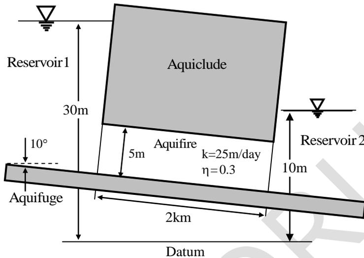
If water in Reservoir 1 is contaminated then the time (in days, round off to one decimal place) taken by the contaminated water to reach to Reservoir 2 will be \_\_\_\_\_.
