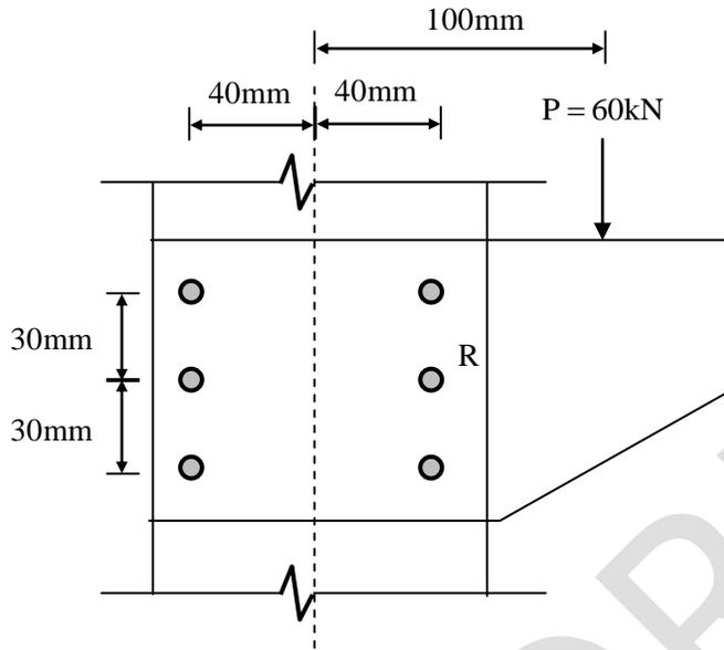
The result force in bolt R (in kN, round off to one decimal place) is \_\_\_\_\_.
