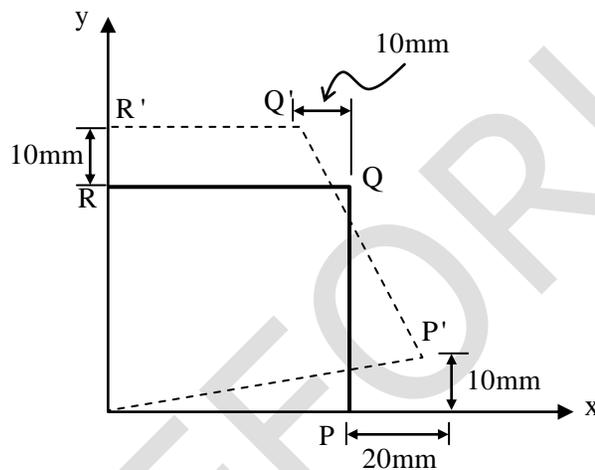
The horizontal displacement of the point (0.5m, 0.5m) in the plate O-P-Q-R (in mm, rounded off to one decimal places) is \_\_\_\_\_.
