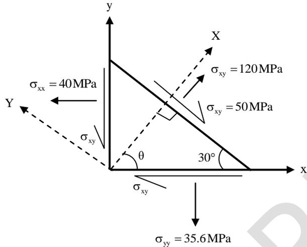
The absolute magnitude of the shear stress component  $\sigma_{xy}$  (in MPa, rounded off to one decimal place) in x-y coordinate system is \_\_\_\_\_.
