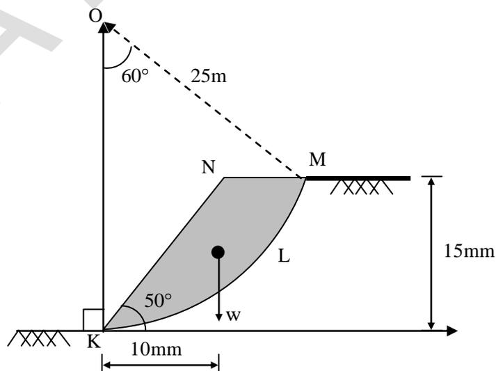
The slope material comprises purely cohesive soil having undrained cohesion 75kPa. A trial slip circle KLM, with a radius 25m, passes through the crest and toe of the slope and it subtends an angle  $60^\circ$  at its center O. The weight of the active soil mass (W, bounded by KLMN) is 2500 kN/m, which is acting at a horizontal distance of 10m from the toe of the slope. Consider the water table to be present at a very large depth from the ground surface.
