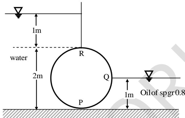
The absolute ratio of the net magnitude of vertical forces to the net magnitude of horizontal forces (rounded off to two decimal places) is \_\_\_\_\_.
