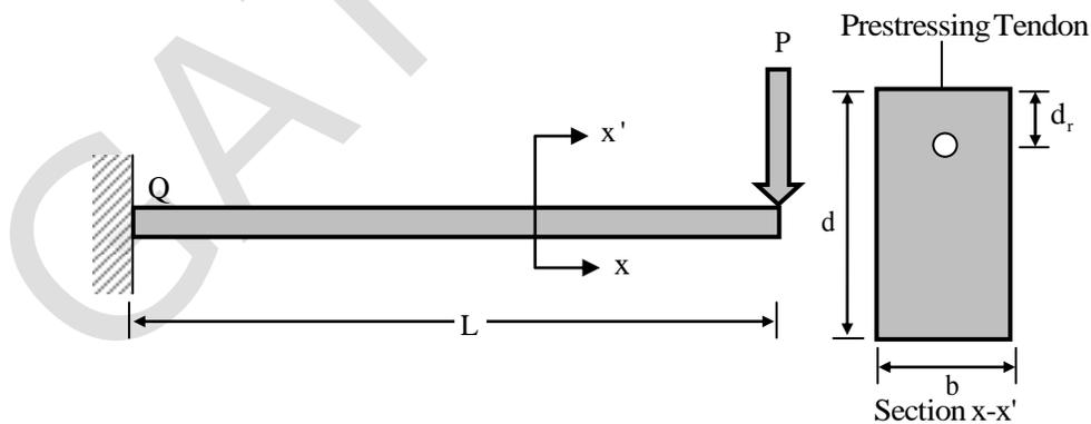
If the concentrated load,  $P= 5\text{kN}$ , the resultant stress (in MPa, in integer) experienced at point 'Q' will be \_\_\_\_\_.
