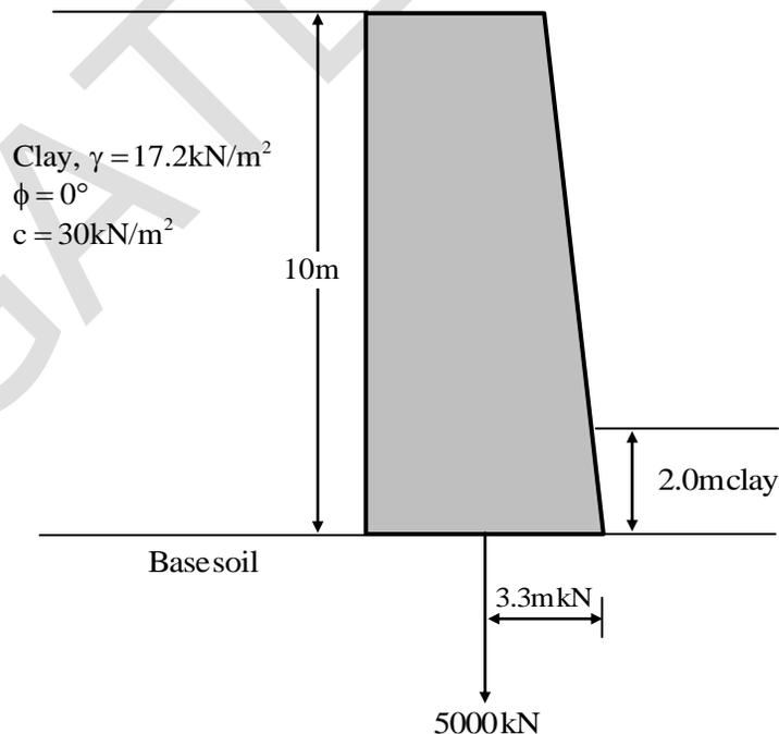
The factor of safety (Rounded off to two decimal places) against sliding failure of the retaining wall after ignoring the passive earth pressure will be \_\_\_\_\_.
