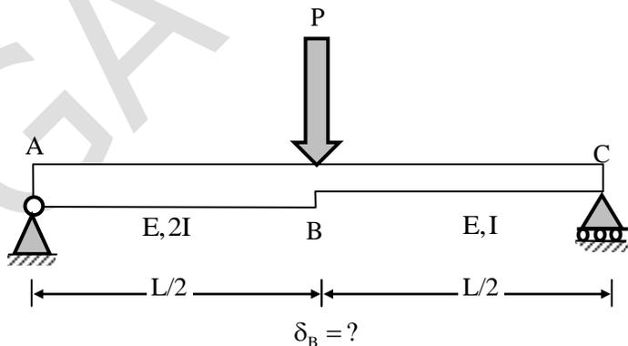
As deflection to be find out at mid span (point load location) strain energy method is the easiest to find.
