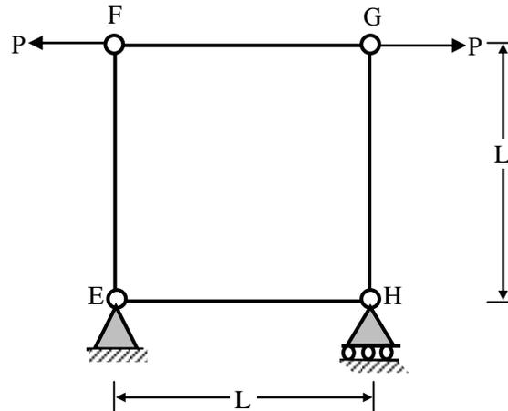
If  $R = 500 \times 10^3 \text{ kN}$ ,  $P = 150 \text{ kN}$  and  $L = 3 \text{ m}$ , the magnitude of the horizontal displacement of joint  $G$  (in mm, round off to one decimal place) is \_\_\_\_\_.
