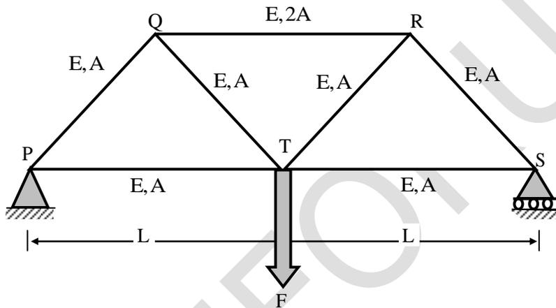
If load,  $F = 10\sqrt{3} \text{ kN}$ , moment of inertia,  $I = 8.33 \times 10^6 \text{ mm}^4$ , area of cross-section,  $A = 10^4 \text{ mm}^2$ , and length,  $L = 2 \text{ m}$  for all the members of the truss, the compressive stress (in  $\text{kN/m}^2$ , in integer) carried by the member Q-R is \_\_\_\_\_.
