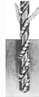
Chip formation of a drill
