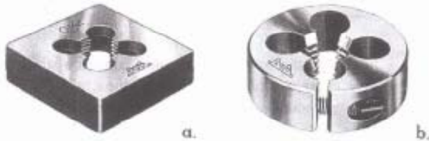
(a) Solid threading die; (b) solid-adjustable threading die
