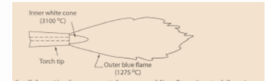
Oxy-acetylene gas welding neutral flame
