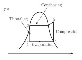
T-s diagram for given Refrigeration cycle is given above Since Heat is extracted in evaporation process.
