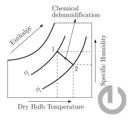
In the process of chemical dehumidification of air, the air is passed over chemicals which have an affinity for moisture and the moisture of air gets condensed out and gives up its latent heat. Due to the condensation, the specific humidity decreases and the heat of condensation supplies sensible heat for heating the air and thus increasing its dry bulb temperature.
