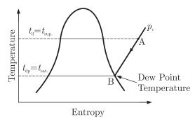
It is the temperature of air recorded by a thermometer, when the moisture (water vapour) present in it begins to condense.
