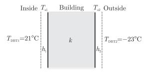
Let  $h_1 \& h_2$  be the internal and external surface heat transfer coefficients respectively and building wall has thermal conductivity k.
