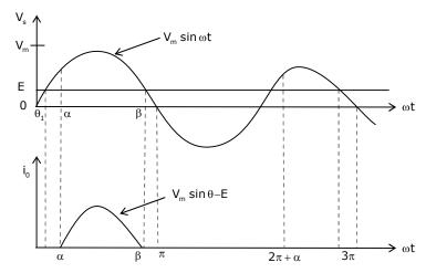
Min firing angle to turn on SCR is Q<sub>1</sub>
