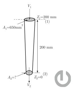
Given :  $A_1 = 650 \text{ mm}^2$ ,  $Q = 6.5 \times 10^5 \text{ mm}^3/\text{sec}$ ,  $g = 10^4 \text{ mm/sec}^2$ Now, for section 1st, flow rate
