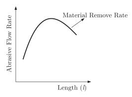
Graph for abrasive jet machining for the distance between the nozzle tip and work surface (l) and abrasive flow rate is given in figure.
