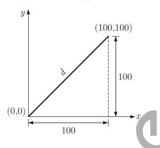
Distance travelled for cut between points (0,0) and (100,100)
