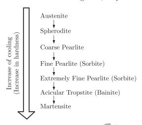
So hardness is increasing in the order, Spherodite → Coarse Pearlite → Fine Pearlite → Martensite
