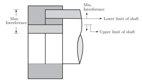
The interference is the amount by which the actual size of a shaft is larger than the actual finished size of the mating hole in an assembly.
