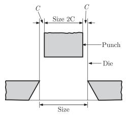
The punch size is obtained by subtracting the clearance from the die-opening size. Clearance is the gap between the punch and the die. (From the figure)
