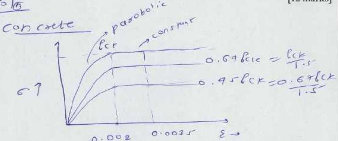
① Stress strain curve of concrete is taken as parabolic rectangular, it validates test results.
