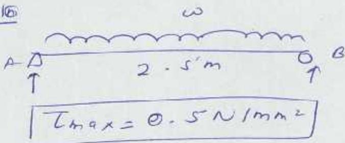
maximum shear stress will be at supports A and B as  $V_{max} = \frac{w l}{2}$
