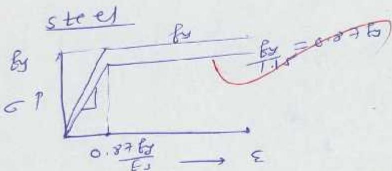
① σ-ε curve is considered straight line upto  $\epsilon = 0.87 f_y / E_s$ , after that stress remains constant only strain increases. Slope till  $0.87 f_y / E_s = \sigma$  is Estd
