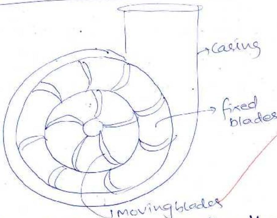
↳ Energy transfer in impeller then the energy transformation in fixed blades.
