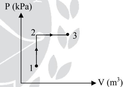
$$\text{Total heat supplied} = m c_v (T_2 - T_1) + m c_p (T_3 - T_2)$$
