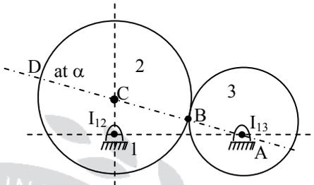
Disc '1' does not rotate about its C.G.
