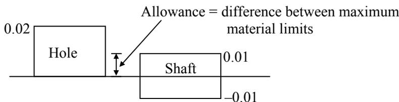
Allowance = difference between MML of hole and shaft
