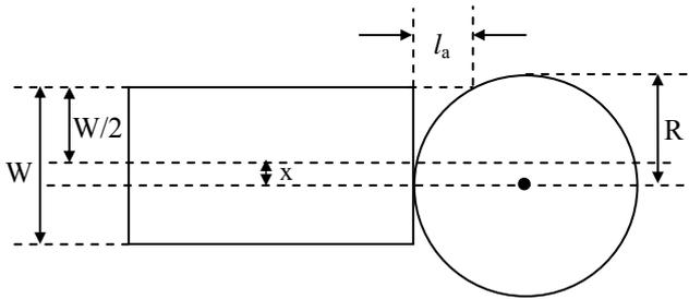
If  $R$  is the cutter radius, ' $W$ ' is the width of the workpiece and ' $x$ ' is the offset, then the length of approach ( $l_a$ ) is expressed as
