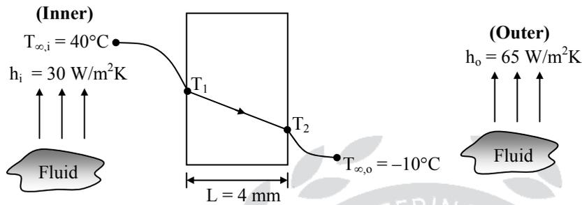
$$\text{Heat transfer rate} = \frac{T_{\infty,i} - T_{\infty,o}}{\frac{1}{h_i A} + \frac{L}{k.A} + \frac{1}{h_o A}} = \frac{T_2 - T_{\infty,o}}{\frac{1}{h_o .A}} \quad (1)$$
